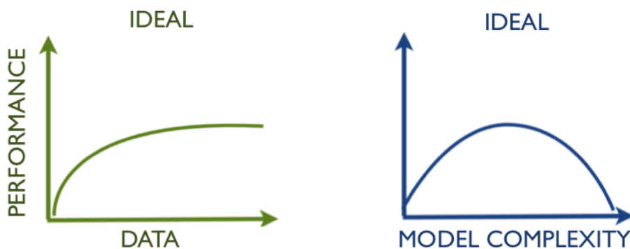
FIGURE 8. Intuitively, we expect the ML model's performance to improve with more data but to deteriorate in performance if the model becomes overly complex for the data. Figure adapted from [317].
